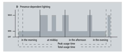
Fig. 6 Energy saving by means of presence-orientated lighting
