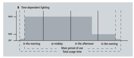
Fig. 3 Energy saving by means of central switching off and time-dependent lighting
