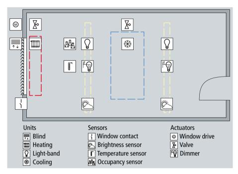
Fig. 4 Units, sensors and actuators for the control of an office
