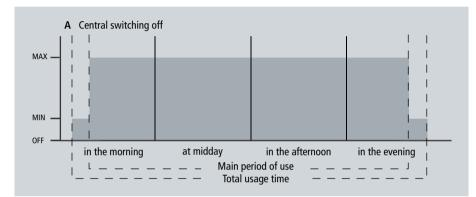
Fig. 2 Saving of energy by central switching off
