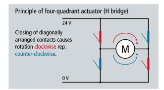
Fig. 3 Four-quadrant actuator
