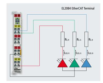
Options for controlling LEDs with Beckhoff EtherCAT and Bus Terminals
