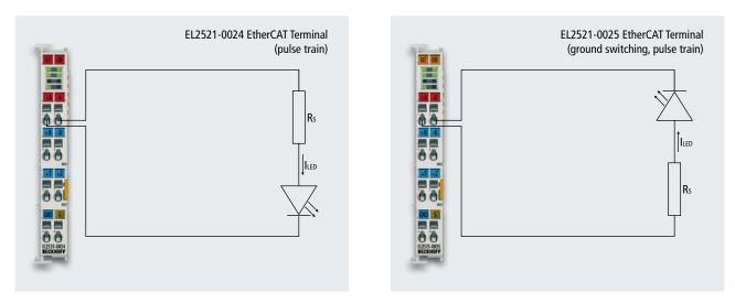
Figure 7: Monochrome LED at a pulsating output
