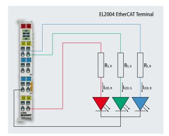
Figure 2: Multicolored LED in voltage mode on standard output
