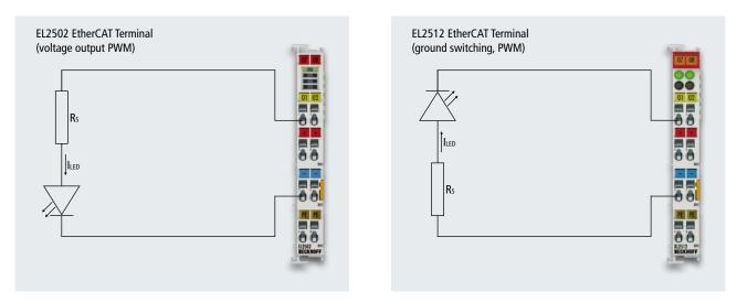
Figure 5: Monochrome LED at a pulsating output
