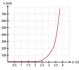
Figure 1: Example characteristic curve of an LED
