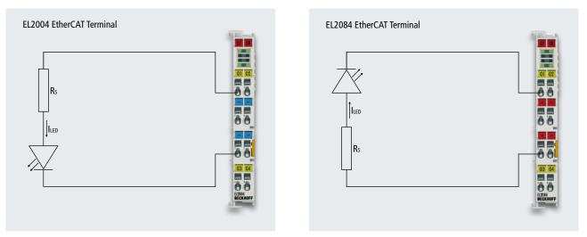
Figure 1: Monochrome LED in voltage mode on standard output
