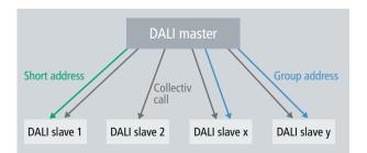
Fig. 4 Addressing the DALI devices via short address, group address or collective call
