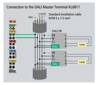
Fig. 6 Power supply via the KL6811 DALI Master Terminal
