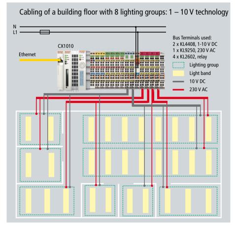
Fig. 10 Cabling expenditure and use of materials with 1 – 10 V technology
