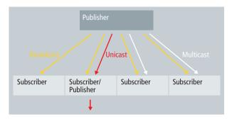
Fig. 1 Broadcast, multicast and unicast as communication modes
