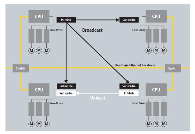
Fig. 5 Multimaster communication via TwinCAT network variables and a real-time Ethernet backbone
