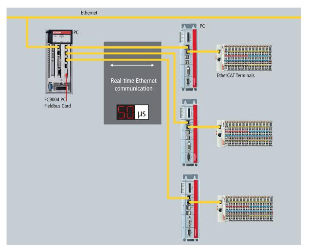
Fig. 7 Ultra-fast communication between several PCs via FC9004
