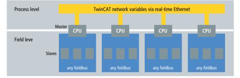
Fig. 4 Different communication channels at the field and process level
