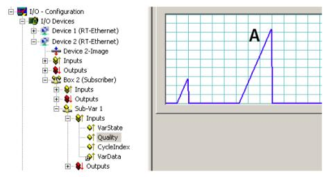
Fig. 2 TwinCAT System Manager with diagnostic function for viewing the latency times of the individual variables.
