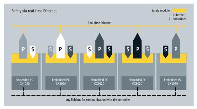
Fig. 6 Distributed Safety via real-time Ethernet within a modularised production line
