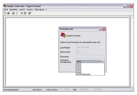
Fig. 3 Access to the virtual COM port through applications/programs (e.g. HyperTerminal)
