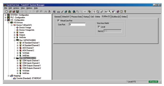
Fig. 2 Numbering of the virtual COM port in TwinCAT System Manager
