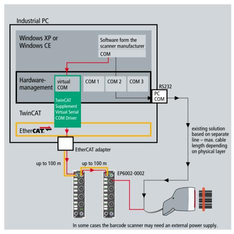
Fig. 4 Connecting a scanner
