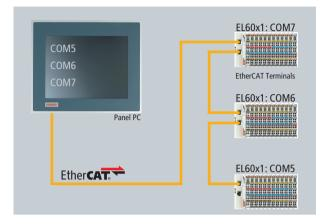
Fig. 1 Serial interface in the field
