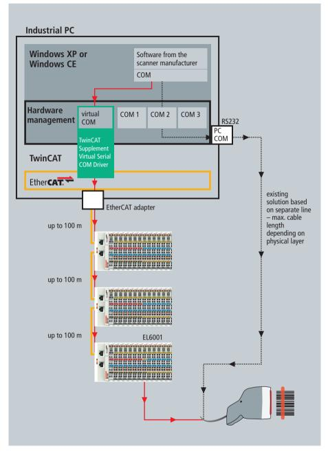
Fig. 2 Connecting a scanner
