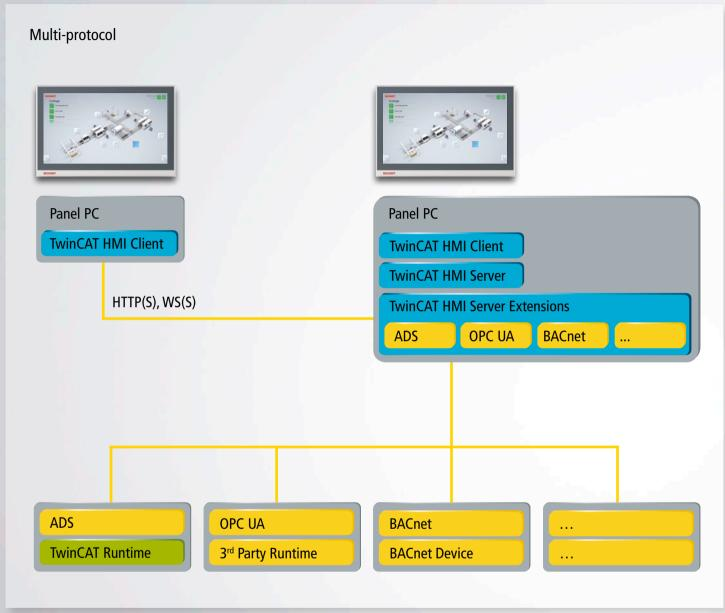
The TwinCAT HMI server can use several protocols in parallel.
