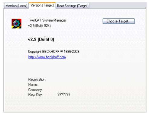
**Choose Target:** Calls the selection dialog for TwinCAT target systems, accessible by TwinCAT Router. See also:Main Menus -> "Actions"
