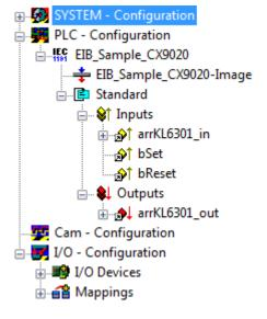
Now link the global variables of the PLC program with the Bus Terminal inputs and outputs, create the allocations, and activate the configuration. Then start the device in run mode. Your CX is now ready for use.
