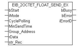
This function block sends a 2-byte float EIB value to the set group address. An IEC61131-3 real value is available as input value. In dependence of the mode (*iMode*) the data can be sent manually, by polling or on change.
