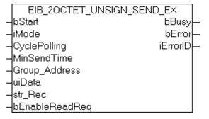
This function block sends a 2-byte Unsign EIB value to the set group address. An IEC61131-3 UINT value is available as input value. The data can be sent in Manual, Polling or OnChange depending on the set mode (*iMode*).
