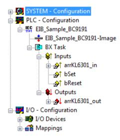
Now link the global variables of the PLC program with the Bus Terminal inputs and outputs, create the allocations, and activate the configuration. Then start the device in run mode. Your BC is now ready for use.
