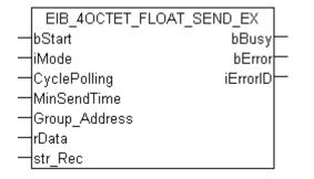
This function block sends a 4-byte float EIB value to the set group address. An IEC61131-3 real value is available as input value. In dependence of the mode (*iMode*) the data can be sent manually, by polling or on change.
