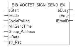
This function block sends a 4-byte sign EIB value to the set group address. An IEC61131-3 DINT value is available as input value. In dependence of the mode (*iMode*) the data can be sent manually, by polling or on change.
