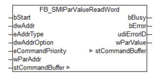
Reads a Word parameter (2 bytes) stored on the motor side. The meaning of the individual parameters is manufacturer-specific.
