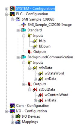
Now link the global variables of the PLC program with the Bus Terminal inputs and outputs, create the allocations, and activate the configuration. Then start the device in run mode. Your CX is now ready for use.
