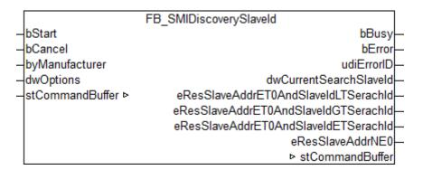
The first drive is sought that corresponds to the specified manufacturer code and has the address 0. This function block is used in the addressing of SMI devices and is used in the FB SMIAddressing [▶ 42] block.
