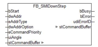
Motor operation downwards by a specified angular degree (0-510 degrees).
