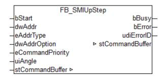
Motor operation upwards by a specified angle (0-510 degrees).
