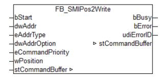
Writes the fixed position *Pos2* which is configurable on the motor side. *Pos2* can be changed using the <u>FB SMIPos2Read()</u> [▶ 34] block.
