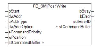
Writes the fixed position *Pos1* which is configurable on the motor side. *Pos1* can be changed using the <u>FB SMIPos1Read()</u> [▶ 30] block.
