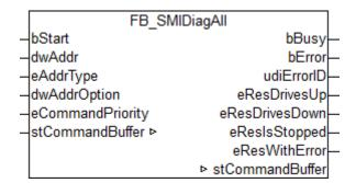
Using this command it is possible to determine the direction in which the drives are driving, whether they have stopped or whether there is a motor error. The command can also be sent also to several SMI slaves. The states of all SMI slaves can thus be queried with a single command.
