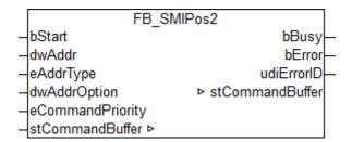
Drives to the fixed position *Pos2* configured on the motor side. The reading and changing of *Pos2* is possible with the <u>FB SMIPos2Read()</u> [• 34] and <u>FB SMIPos2Write()</u> [• 35] blocks.
