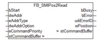
Reads the fixed position *Pos2* configured on the motor side. *Pos2* can be changed using the <u>FB SMIPos2Write()</u> [• 35] block.
