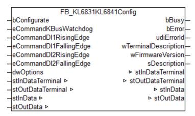
This block is used to configure the KL6831/KL6841. The configuration is executed when the PLC program starts, or it can be triggered by a positive edge at the input *bConfigurate*. The parameters are stored in the respective registers of the KL6831/KL6841 in a fail-safe manner. In addition, some general information, such as the firmware version, is read from the KL6831/KL6841.
