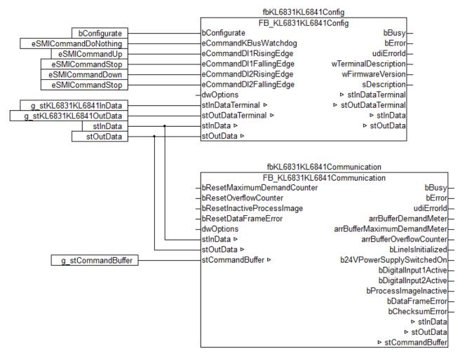
The block FB\_KL6831KL6841Config() is linked to the process image of the KL6831/KL6841. After the configuration, the block FB\_KL6831KL6841Communication() is assigned the process values of the KL6831/KL6841. During the configuration, it is not possible to send SMI commands.
