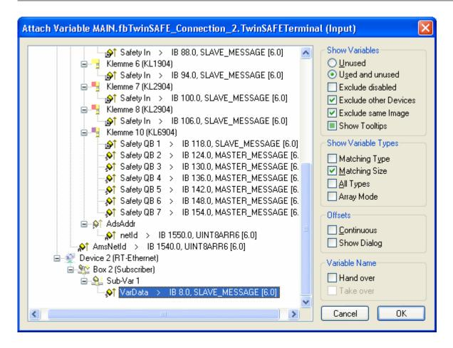
The linkage of the output data of the connection must be done by marking the parameter TwinSAFELogic and choosing "Change Link..." from the context menu and choosing the correct SafetyQBx variable in the upcoming dialog.
