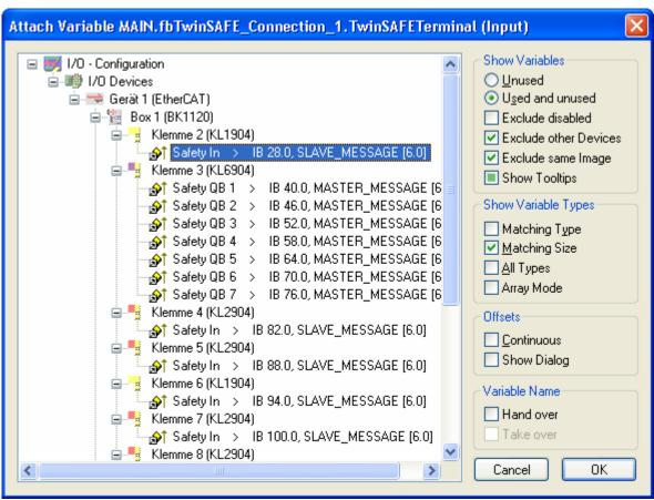
When using RT Ethernet for the TwinSAFE communication please choose the corresponding subscriber variable.
