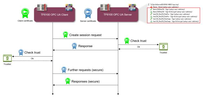
The client transmits its public key with the CreateSession Request. The server then has the option of checking the trust relationship. If the server trusts the client, it transmits its own public key in its response. The client therefore also has the option of checking the trust relationship with the server.
