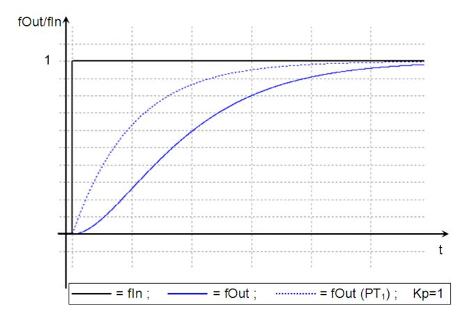
This  $PT_2$  element consists of a series of two  $PT_1$  elements; the time constants T1 and T2 can have different values. The step response (see above) shows a significantly more attenuated subsequent behavior compared to the  $PT_1$  element (dashed) right from the start.
