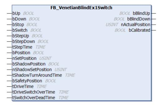
Blind function block with the same functionality as <u>FB\_VenetianBlindEx()</u> [• 23] but with an input *bSwitch* for jogging up and down.
