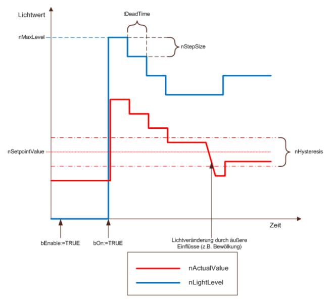
The control is enabled by a TRUE signal at input bEnable. When a positive edge is encountered at bOn, nLightLevel is set to the maximum value. This also influences the measured light value nActualValue, which increases, so that dimming becomes necessary. nLightLevel is now reduced step-by-step until the measured light value nActualValue is in the hysteresis range around the setpoint (nSetpointValue - 0.5\*nHysteresis < x < <math>nSetpointValue + 0.5\*nHysteresis).
