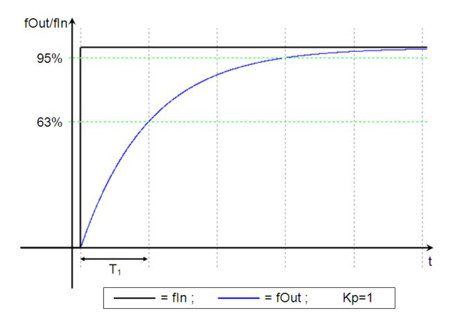
If Kp is 1 the output value directly follows the input value. *fOut has* reached 63% of the input value after the time tT1 has elapsed, after 3 x tT1 the value is 95%.
