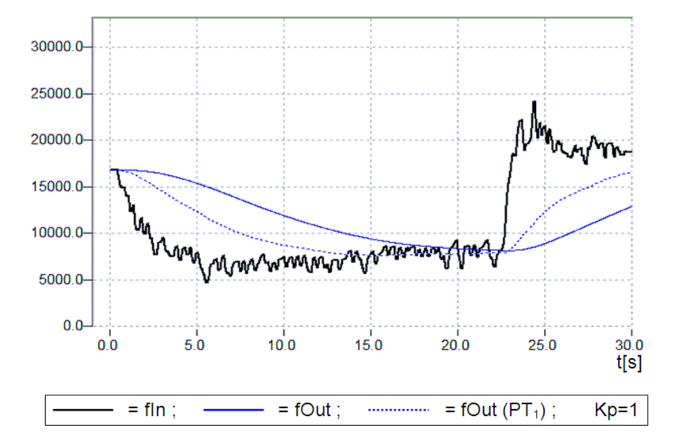
In comparison, the dotted line shows the behavior of a <u>PT1 element [ $\triangleright$  28]</u> with *fln*= 0..33000, *Kp*= 1, *T1*= 5s.
