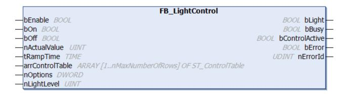
Function block for daylight-dependent lighting control with up to 30 interpolation points.
