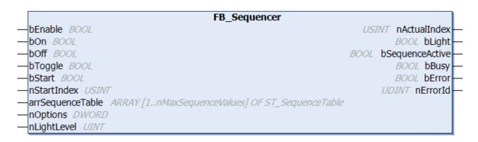
Function block for realizing light sequences with up to 50 interpolation points.
