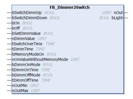
The function range of the function block corresponds to that of the function block <u>FB Dimmer1Switch()</u> [> <u>37]</u>. The difference is that in the function block FB\_Dimmer2Switch two switches are connected. This allows the user to choose specifically between dimming up or dimming down.
