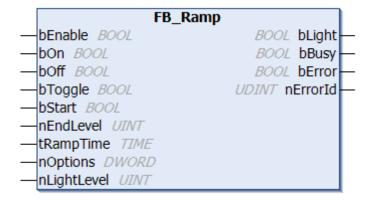
Function block for realizing a light-ramp.
