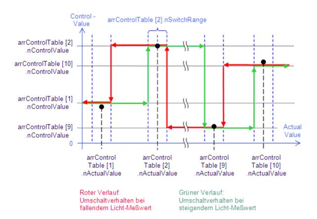
The whole range of the table does not have to be used. The first table element (*arrControlTable*, see below) for which the parameter *nSwitchrange* is 0 is considered the start of the unused area.
