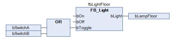
If either the *bSwitchA* or the *bSwitchB* button is pressed, then the state of the light, as represented by the *bLight* output, is changed.
