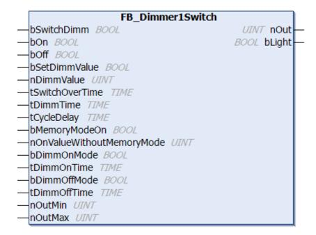
The function block is used to dim lights with a switch.
