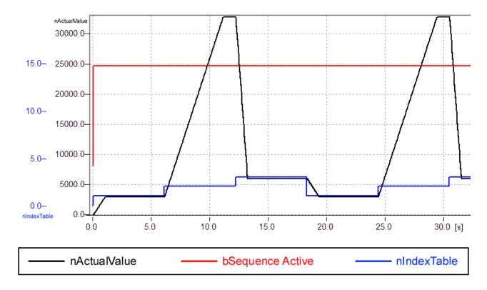
In addition, the function block can be switched on and off "normally" (On: nLightLevel = 32767, Off: nLightLevel = 0) or toggled between "On" and "Off" via the input bToggle. However, none of the command inputs is active unless the bEnable input is TRUE. If it is reset to FALSE, no more commands are accepted and the light value retains its current state – even from a ramp.
