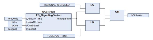
The following example illustrates the simplest case. A message signal not requiring acknowledgement.
