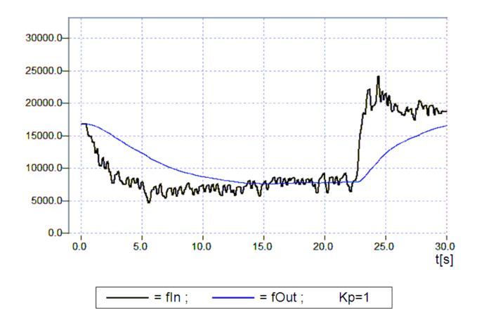
Note on damping times: Since this function block is a time-discrete model of a PT<sub>1</sub> element, it only works correctly if the damping time is significantly longer than the set cycle time. To be on the safe side, if a damping time is entered that is less than twice the set cycle time it is internally set to zero. A damping time of 0s means that the output variable directly follows the input variable multiplied by Kp.
