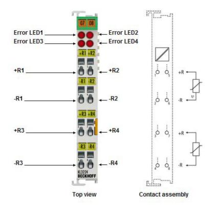
Fig. 12: KL3224 - connection and LEDs
