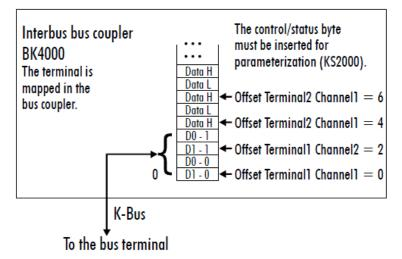
Fig. 16: Mapping in the Interbus coupler – example for KL3202
