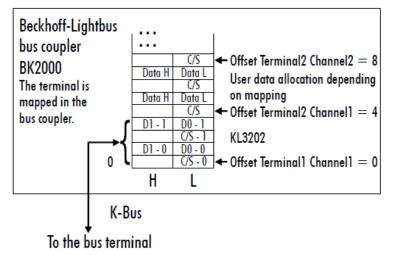
Fig. 14: Mapping in the Lightbus Coupler\_KL3202
