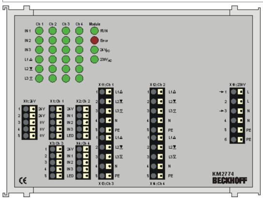
Fig. 3: KM2774 - Wiring
