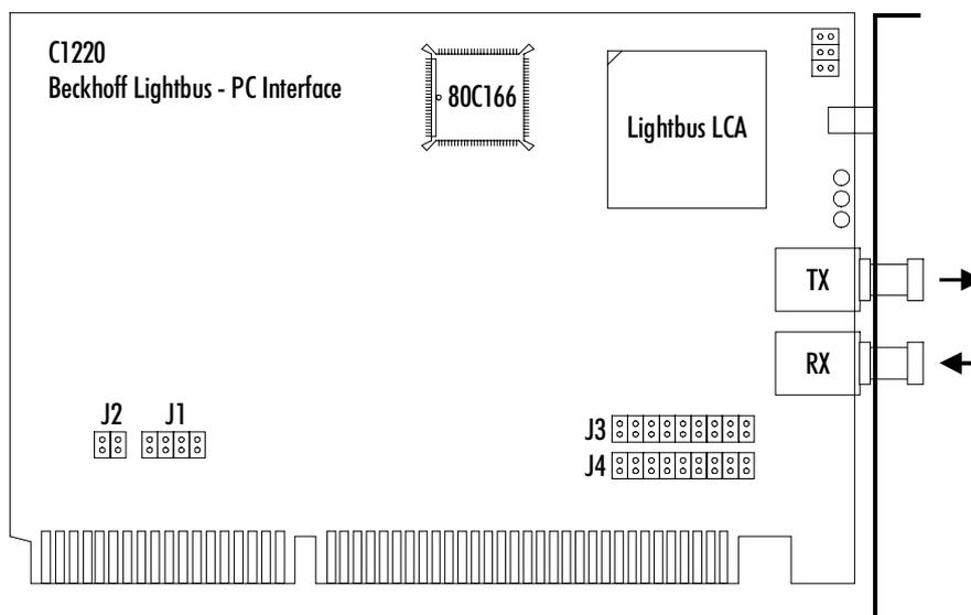
The Lightbus - PC interface C1220 is an intelligent Lightbus central module.
