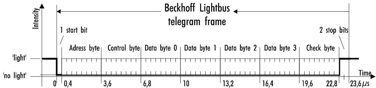
The telegram frame is required for serial, asynchronous data communication and consists of 1 start bit, 6 CRC check bits and 2 stop bits. The telegram frame is generated and checked by the hardware. Software support is not necessary.
