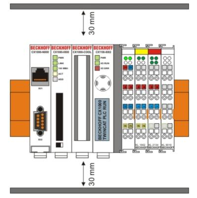
FIG. 8: Allowable installation position
