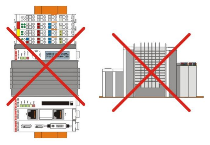
FIG. 9: Allowable installation position
