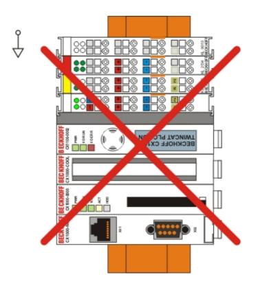
FIG. 10: Unallowable installation position
