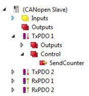
Fig. 63: Diagnostic variable SendCounter of a CANopen slave.
