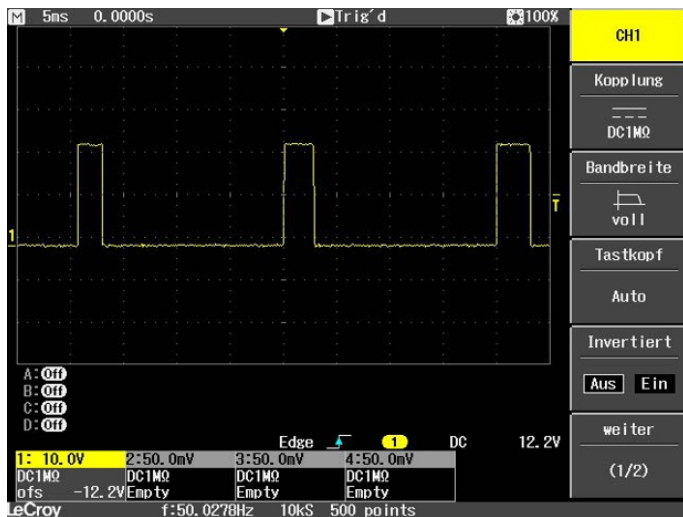
Fig. 41: Shortened pulse of a digital output with load.
